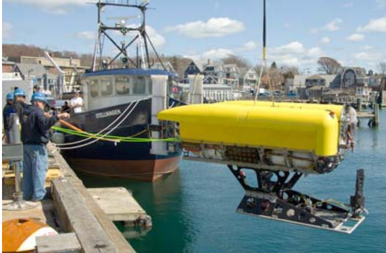
Figure 1: A deep-sea robotic hybrid vehicle
